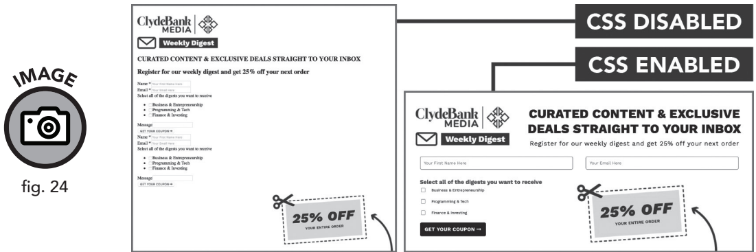
A portion of the ClydeBank Media website with CSS disabled (left) and enabled (right)
